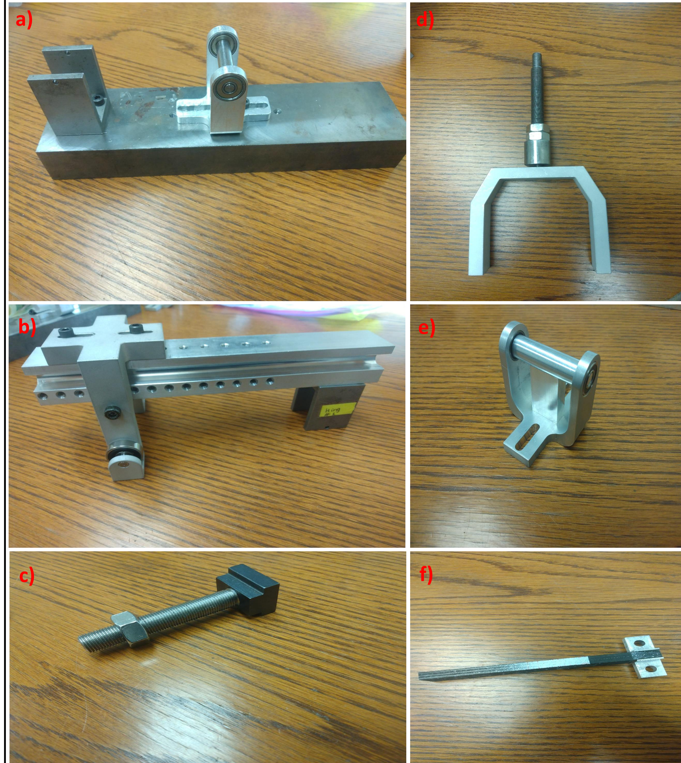
Recently Patented Fabricated MRMMB Components To Be Utilized For Experimental Testing a) Base, Bottom Hinge and Bottom Roller b) Lever, Saddle, Top Hinge c) Base Slider d) Connecting Rod and Yoke e) Top Roller f) Laminated Composite Specimen
