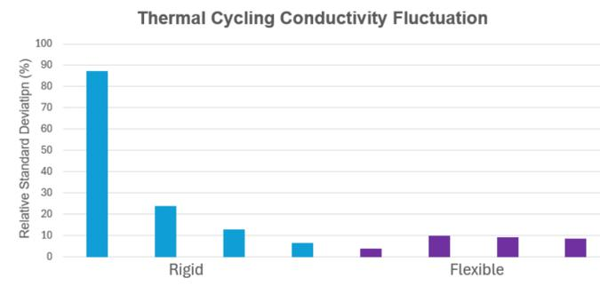
Figure 3. Comparisons between Flexible and Rigid Perovskite Solar Cells were made using Relative Standard Deviation to determine stability. As seen below, averages of the flexible substrates maintained a lower overall conductivity variance, proving a better stability over the course of 200 thermal cycles.
