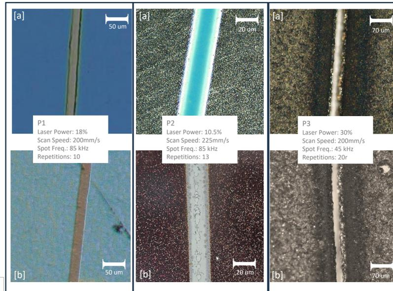
Figure 2. The three different patterning scribes are seen above, with [a] displaying the rigid substrate results, and [b] displaying the flexible. Multiple trial and errors led to the conclusion that, with the layers being of equal width besides substrate, that the scribing power, speed, frequency and repetition were identical.
