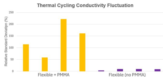
Figure 4. Similar to the figure above, comparisons were then made between the flexible substrates with and without PMMA. Results remained consistent with what was the expected outcome, in which the PMMA created much less stable PSCs, likely due to the reaction that occurred with the Carbon top layer.
