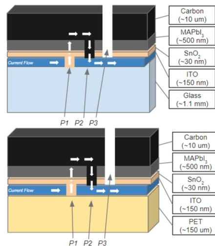
Figure 1. Depiction shows the contents of the MAPI Perovskite Solar Cell that was created for both Rigid (Glass) and Flexible (PET) substrates. Labels for each scribe and their designated current flow are given.
