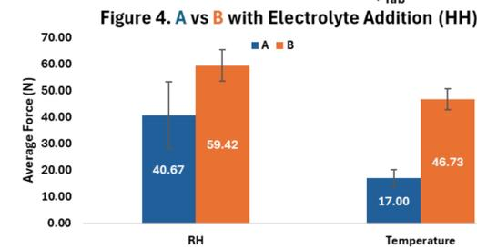
Figure 1 & 2: Average max force of different orientations are shown for materials A and B with comparison of RH and temperature effect. Material B also shows as is (no condition).
