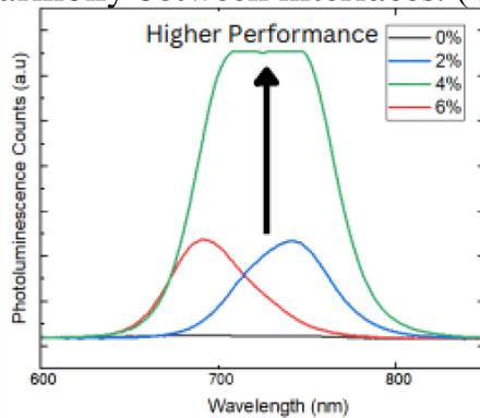
From previous work done it can be seen that Propane-1,3-diammonium iodide with 4% PVP has the highest efficiency, which was the motivation to work on them during this experiment. (Gokce, Berrak)
