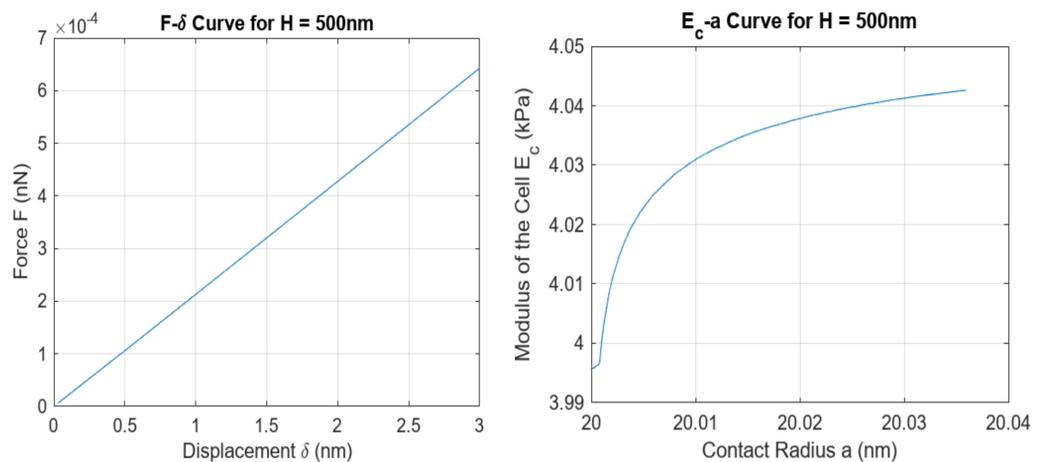
**Fig. 5** Force-displacement curve for cell with height of 500 nm (left), load and unloading curves together. Measured elastic modulus vs. contact radius (right) of same indentation test.
