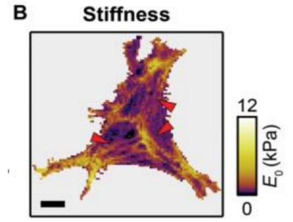
**Fig. 2** Stiffness of a cell in different regions. Measured by AFM. - Schierbaum et. al. 2019
