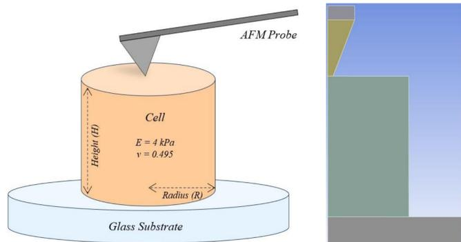
**Fig. 3** Experimental setup (right) and FEA setup for cell with height of 500 nm (left).
