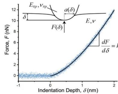
**Fig. 1** Force-displacement curve example and geometry of AFM indentation. - Collinson et. al. 2021
