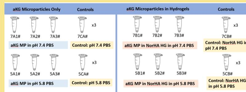
Figure 3: We evaluated the release kinetics for 10 mg of paKG MPs alone and encapsulated within HA hydrogels at a pH of 7.4 and 5.8.
