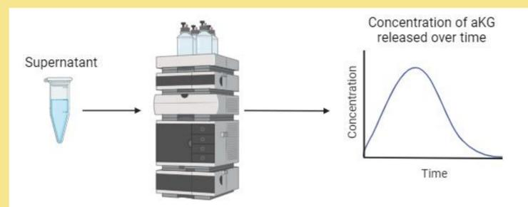
Figure 4: Release supernatant was collected over a 4-week period. High-performance liquid chromatography (HPLC) will be used to determine the concentration of aKG in the supernatant at various time points across the 4-week period.
