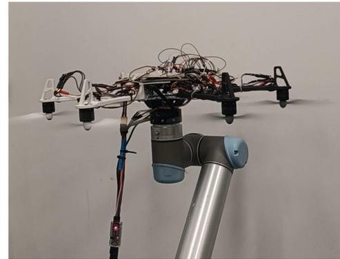
Fig. 3. Experiments setup for Ground Effect
