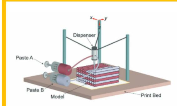
J2027LV, a phenolic resin is used that is known to have high carbon content<sup>3</sup>. We yielded about 60% carbon yield post pyrolysis. Hyrel 3D printer is used for printing. Post-printing, the sample must be kept inside a
