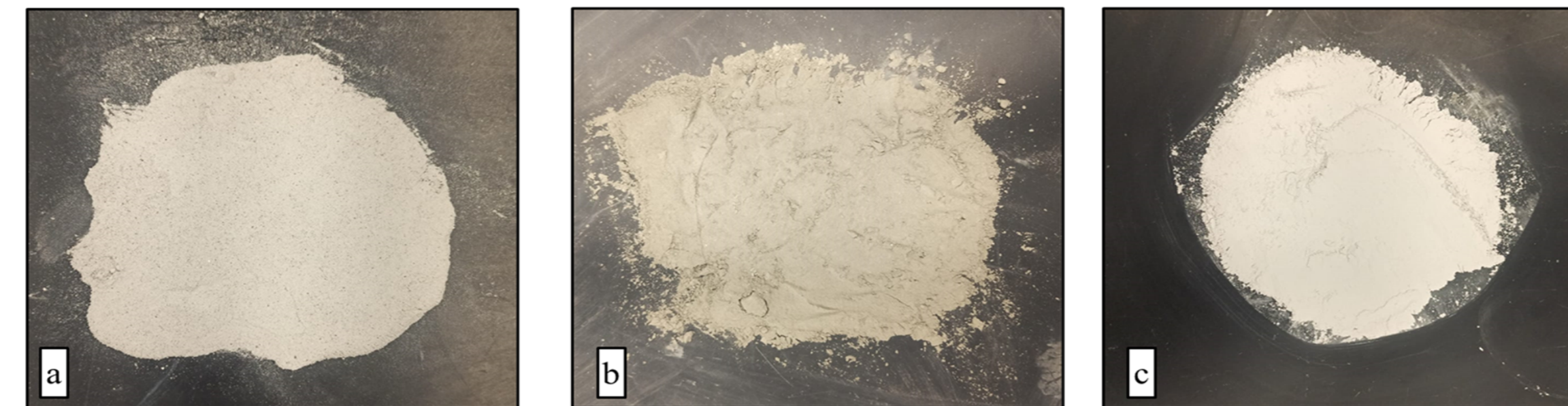
Figure 3: Binders used in the study: (a) mine tailings, (b) cement, and (c) slag
