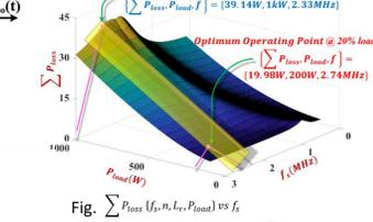
Fig.  $\sum P_{loss} \{f_s, n, L_r, P_{load}\} \text{ vs } f_s$
