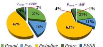
Fig. Loss distribution at light loading and heavy loading operations
