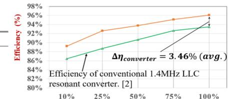
Fig. Efficiency at different loading conditions
