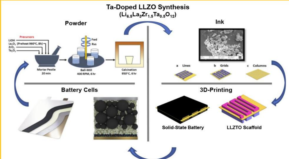
Each different patterning will be tested to determine the performance behavior of our SSE batteries. We hypothesize the ionic conductivity may increase based on uniform shear stress from the patterns [4]. Also, different patterns may be tailored for blocking dendrite propagation which will create stability and have higher energy density.
