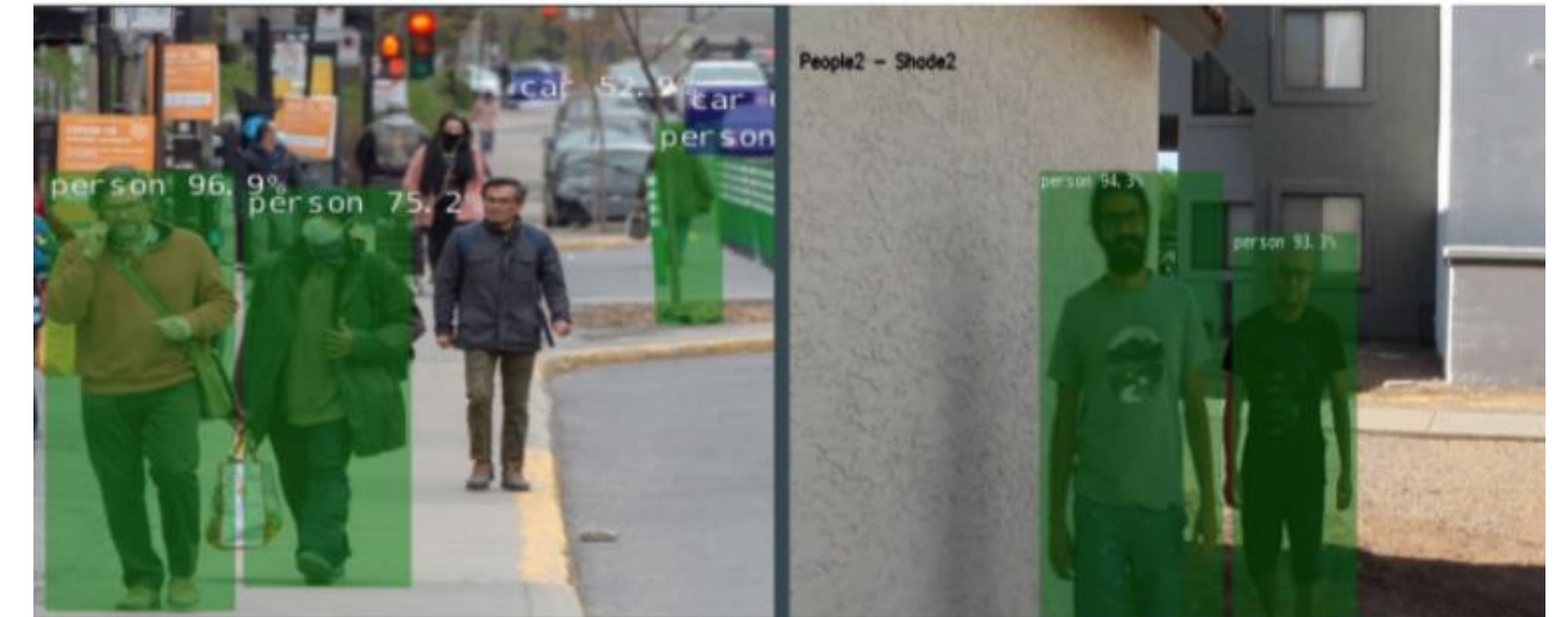
Fig 4: People Counter detecting people (left); counting number of people in shade (right).
