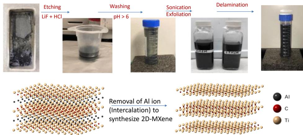
Fig. 1- (a) MAX Phase (b) in-situ HF + MAX phase (c) 2D MXene flakes after intercalation. (d) Sonicated solution with 2D flakes delaminated (e) pure 2D-MXene solution in DI water (f) Microstructure of MAX phase with ions (g) Microstructure of MXene after removal of ions
