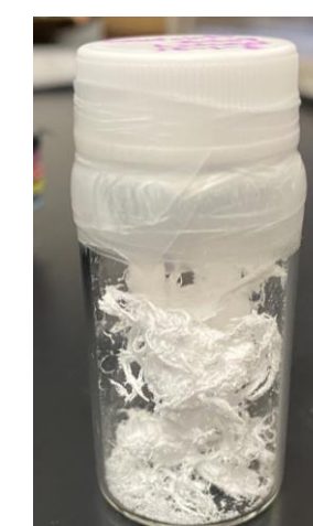
Pure sample (washed with toluene, precipitated in methanol)
