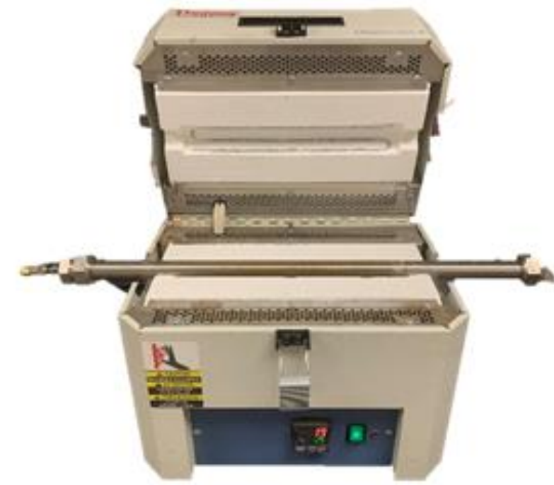
Figure 1: Tube furnace used for sintering
