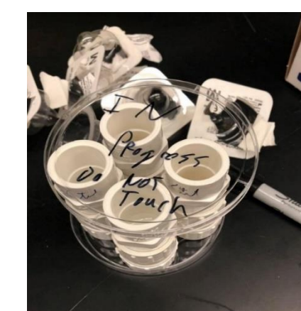
Figure 5: Plastic holders were used to hold RO membranes in place while contacted with P. aeruginosa for 3 hours.
