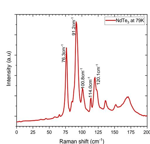
Fig. 2: Raman spectroscopy of NdTe<sub>3</sub> at 79K
