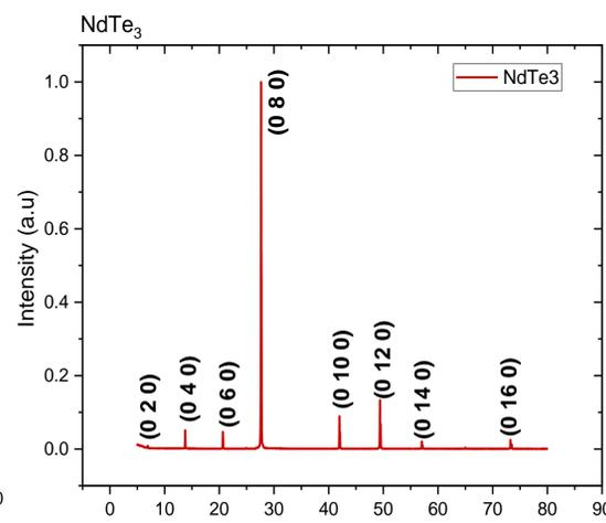
Fig. 3: X-ray Diffraction of NdTe<sub>3</sub> at RT
