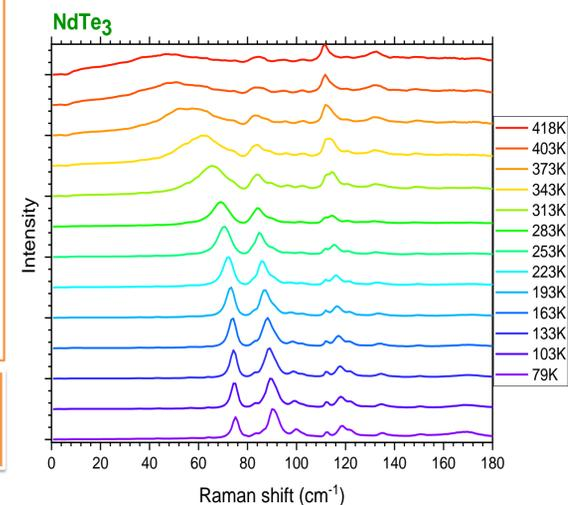
Fig. 3: Temperature dependent Raman spectroscopy of NdTe<sub>3</sub>
