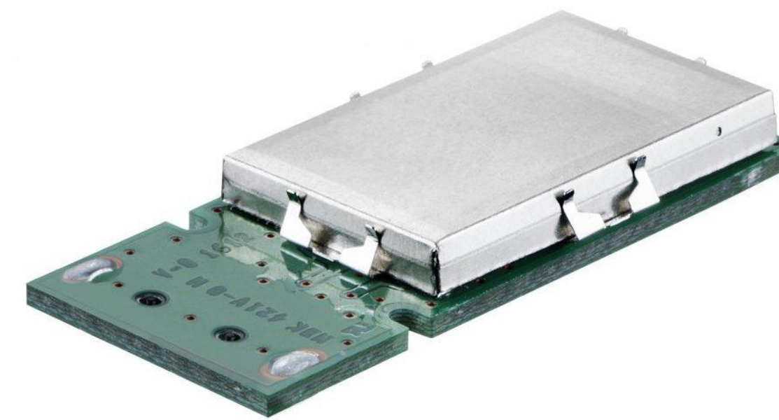
Example of circuit encased in a shielding cabinet.
