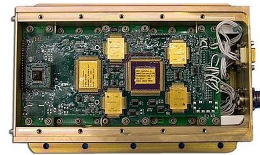
Rad-hardened CMOS memory device for the Radiation Hardened Electronic Memory Experiment (RHEME).
