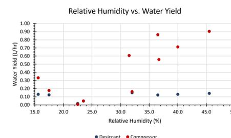
Figure 4. Relative Humidity vs. Water Yield (Liters per hour)
