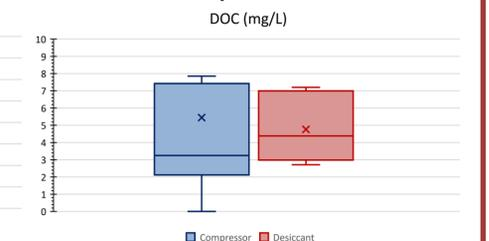
Figure 9. Dissolved Organic Carbon (DOC) for both dehumidifier systems
