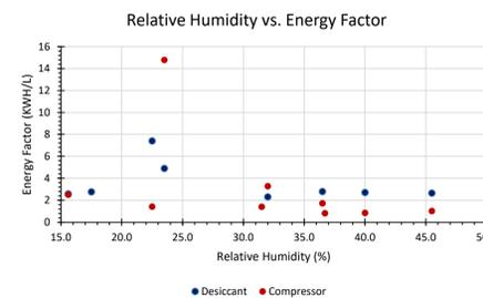
Figure 3. Relative Humidity vs. Energy Factor
