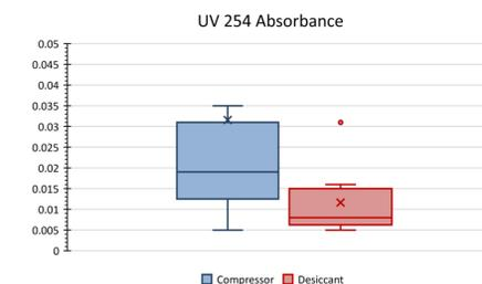
Figure 5. UV 254 absorbance for both dehumidifier systems
