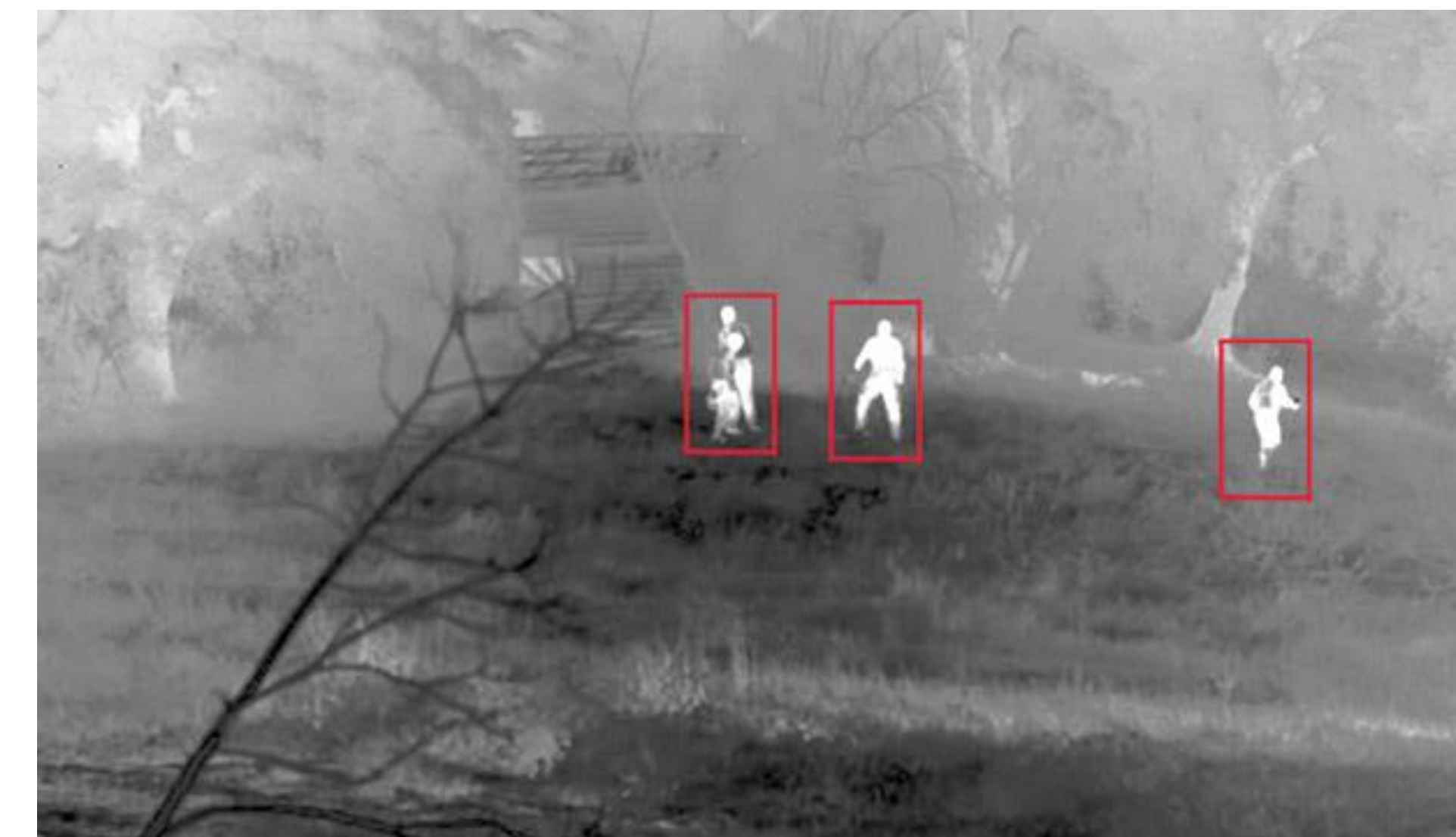
Figure 4. IR Camera in White Hot Mode with People located in Red Box Tracking
