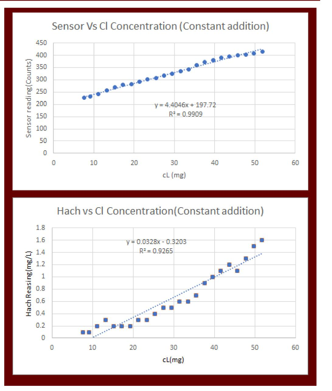
These figures compare the chlorine sensor developed and a market competitor. The chlorine sensor is more precise to a smaller interval and more accurate than the market competitor.
