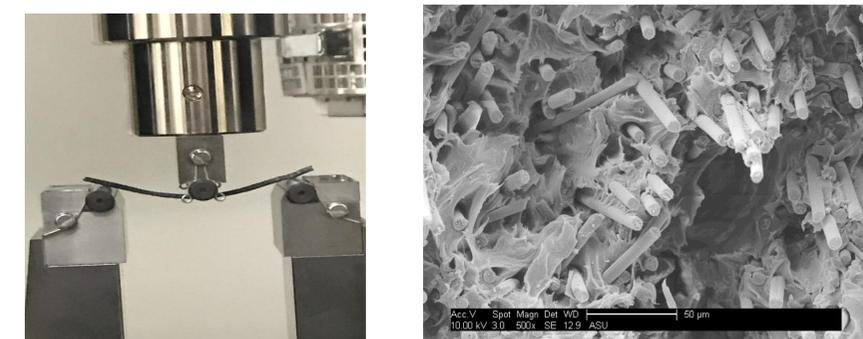
**Targeted composite structures and our composite filaments with carbon fiber alignment. We will use 3-point bending to study the composite mechanics**
