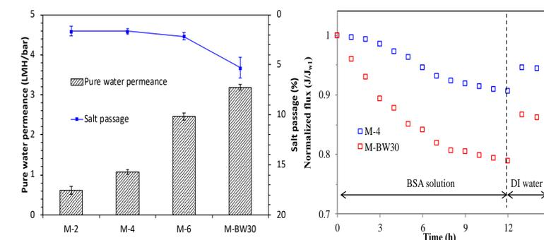
Fig 6: a) Pure water permeance at 8 bar and 25°C with 1 g/L NaCl feed b) Normalized Flux with BSA solution feed and after washing with DI water [6]
