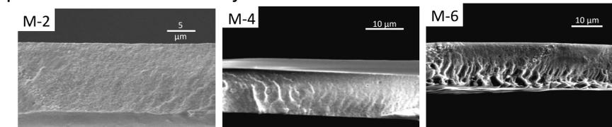
Fig 5: SEM images of cross-sections of M-2, M-4 and M-6 membranes
