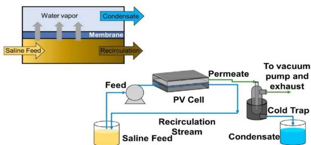
Fig 2: Schematic of pervaporation setup
