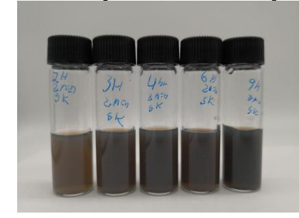
2,3,4,6,9 hr sonication time B<sub>4</sub>C Nanosheets in solution
