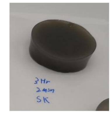
3 hr sonication time  $B_4C$  Nanosheets in hydrogels. Centrifuge process was done at 5000rpm for 2 minutes to gather nanosheets.
