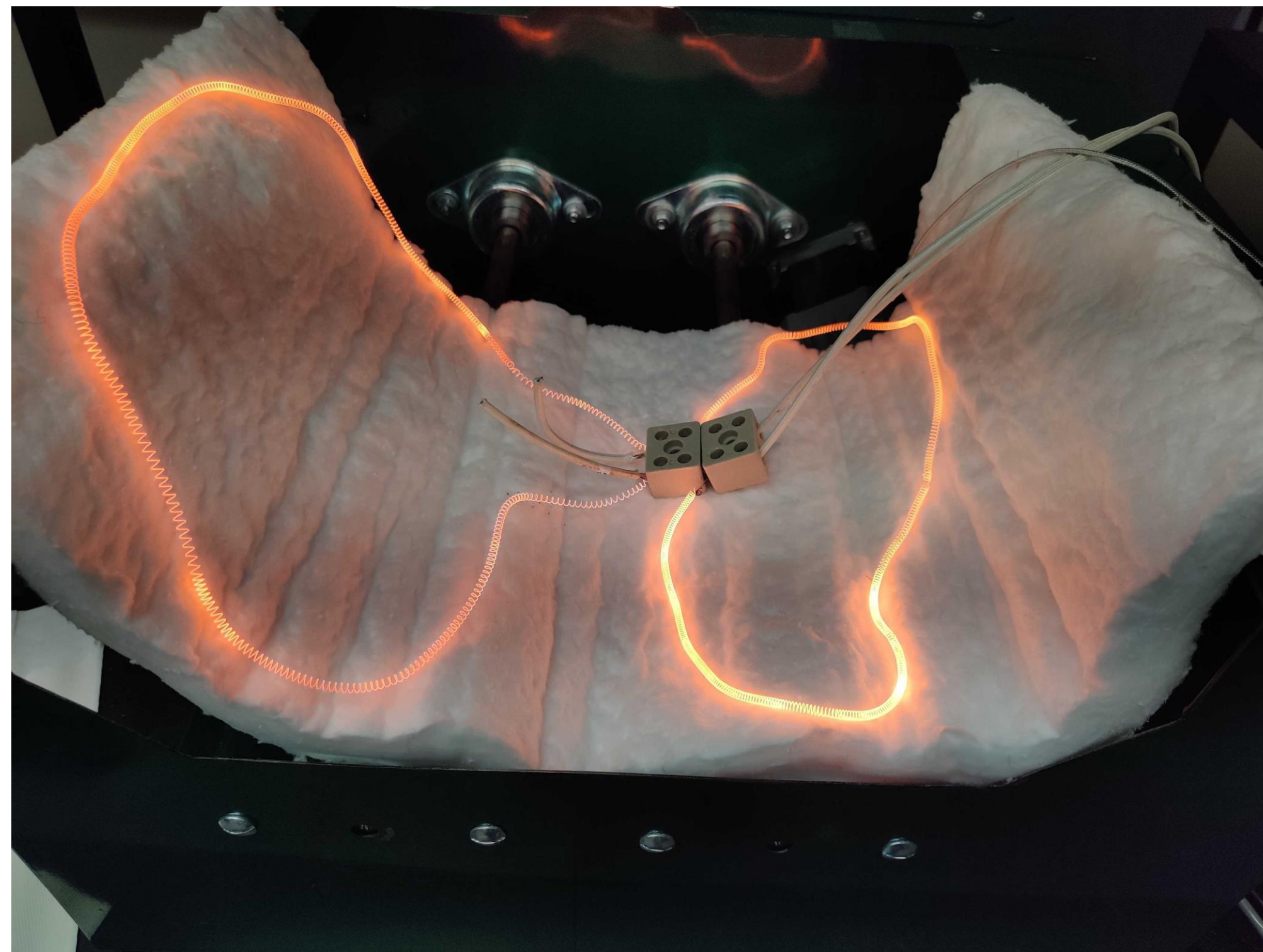
Figure 1. Working Heated Wiring Loop
