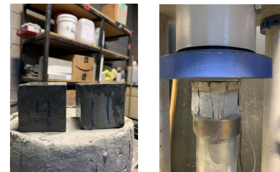
Figure 1. Scenario 1 and 4 mortar cubes before and during compression testing.
